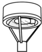
Recessed (flush mounted) Under Canopy Fixture
