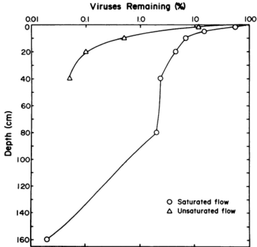
FIG. 1. Virus adsorption by a soil column during saturated and unsaturated flow. Saturated flow points are averages for three infiltration rates, and unsaturated flow points are averages for two infiltration rates.
