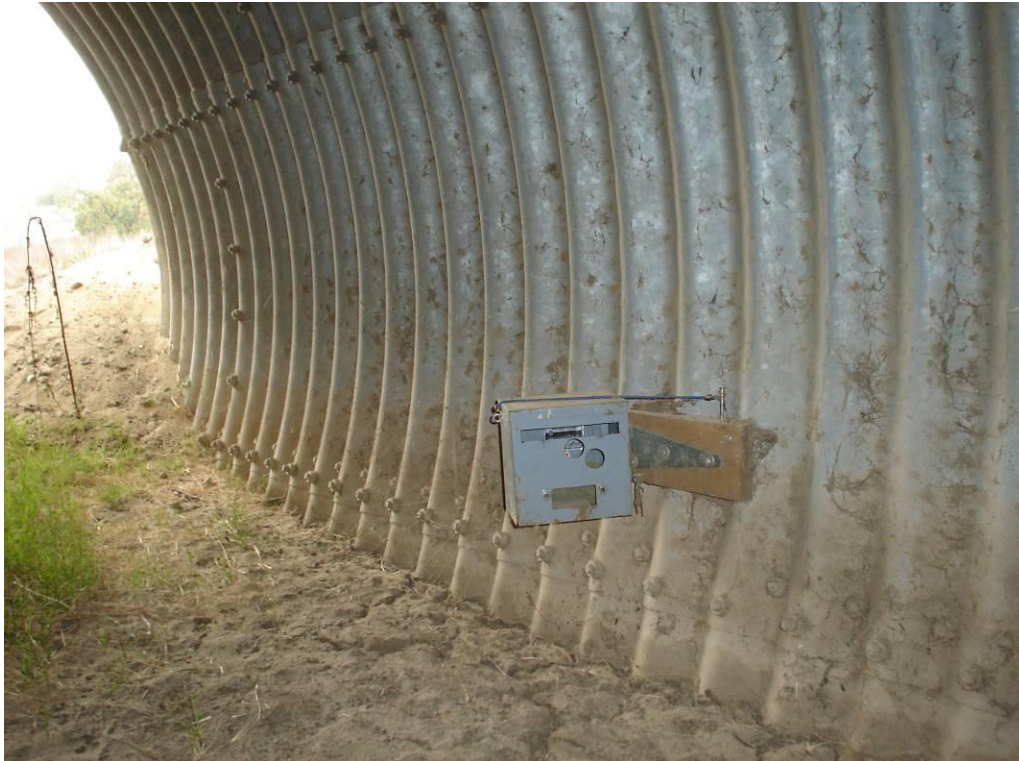
Figure 7. Digital remote camera secured in steel container used to monitor culvert use.
