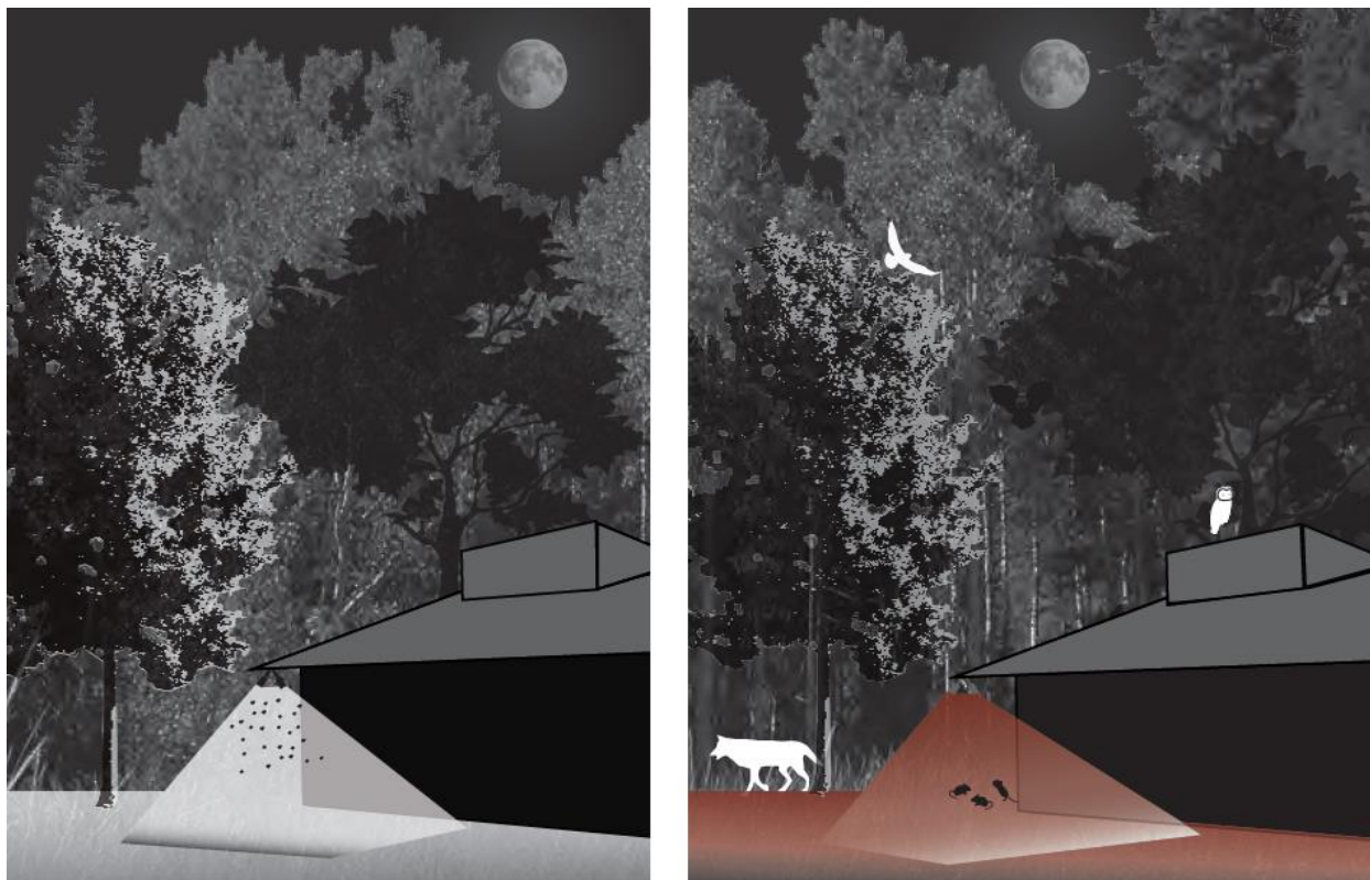
Figure 20. Red light does not disrupt dark-adapted vision and is therefore appropriate for campsites and locations used for astronomical observation.
