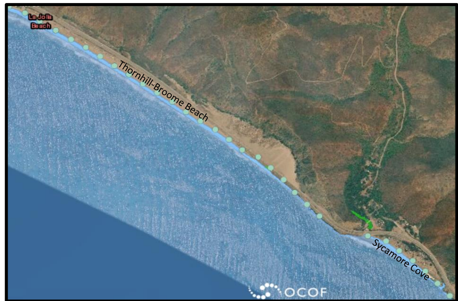
Figure 2-14. Tidal inundation along the Thornhill-Broome Beach and Sycamore Cove area at Point Mugu State Park with approximately 16 inches of sea level rise according to CoSMoS (top). The Coastal Resilience model shows tidal inundation with about 5 feet of sea level rise (bottom).
