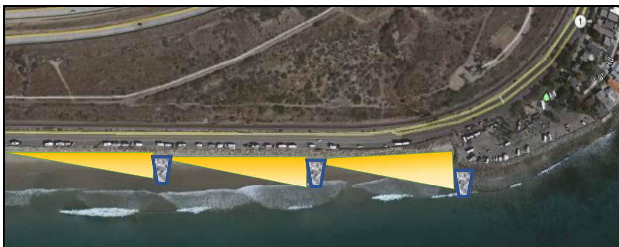
Figure B-8. Map view of cross-shore cobble groins with retained sand on the Rincon Parkway and at Faria County Beach Park (not to scale).
