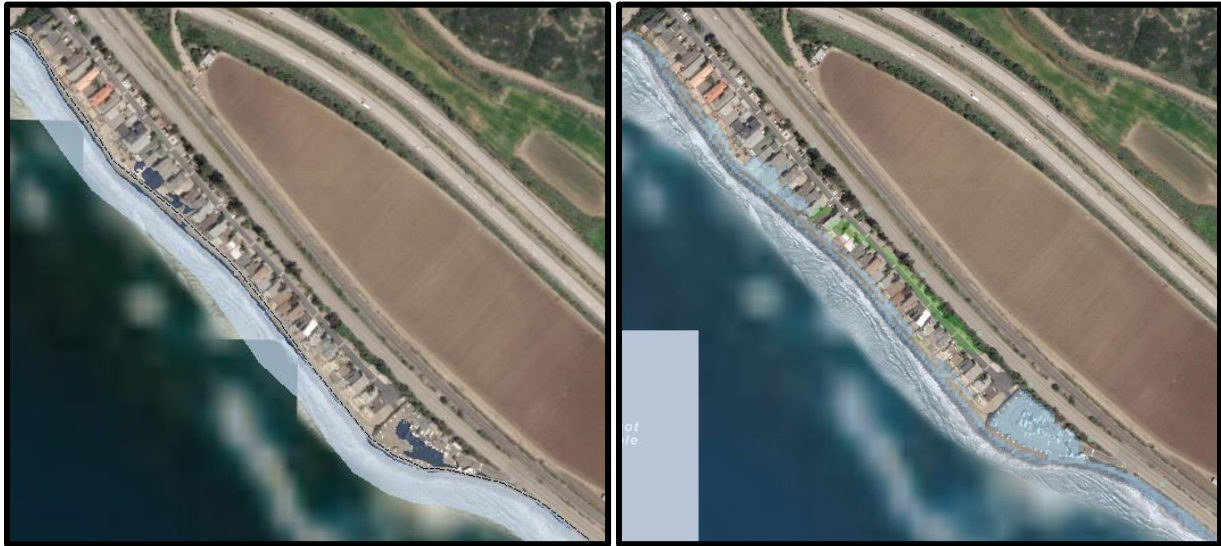
Figure 2-3. Tidal inundation with about 5 feet of sea level rise in Seacliff according to Coastal Resilience (left) and CosMoS (right). The green-colored areas are low-lying areas that could be flooded but are not connected to the shoreline or there is an obstacle blocking the flow.
