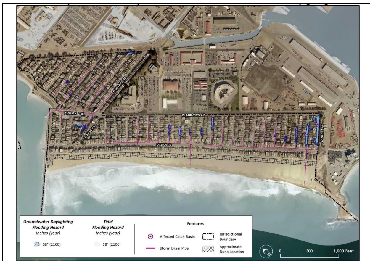
Figure B-5. Potential locations of groundwater daylighting and stormwater induced flooding with 58" of sea level rise.
