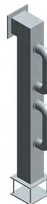
3 POST / WALL RAPPELLING TIE OFF TYPE 2 AXON NOT TO SCALE
