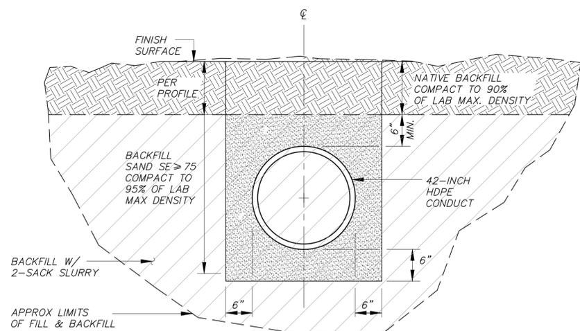
**TYPICAL PIPE INSTALLATION DETAIL I** (B)
