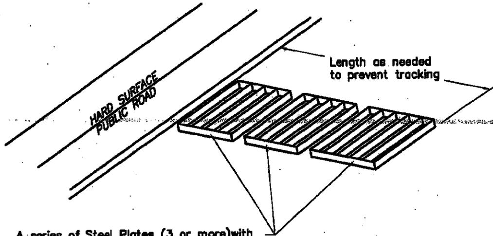
A series of Steel Plates (3 or more) with Rumble Strips or min 4" coarse aggregate.
